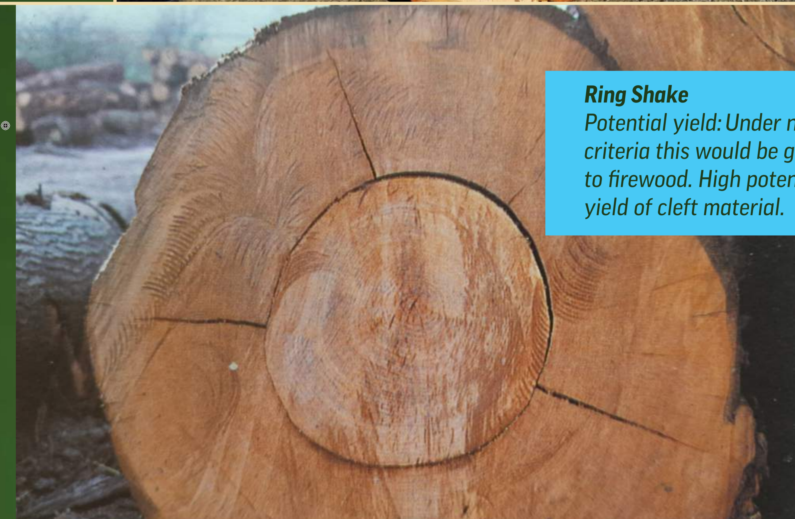
Ring Shake Potential yield: Possible yield of character grade wood from inner section. N.B. Frequent shake in outer rings. It's likely there was a change in soil hydrology, maybe local drainage, that produced severe moisture deficit.
